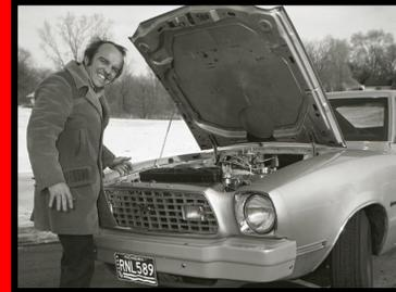
Jack Roush & Wayne Gapp equipped this car with a 505CI Lincoln big block, built Ford C6, narrowed 9 inch rear, 29.5 inch slicks, roll cage and racing seats. Roush also replaced the rear suspension with a fabricated rear sub-frame. Look for this car on TV in an upcoming edition of Dennis Gage's, "My Classic Car", as well as well-known Mustang magazines.
